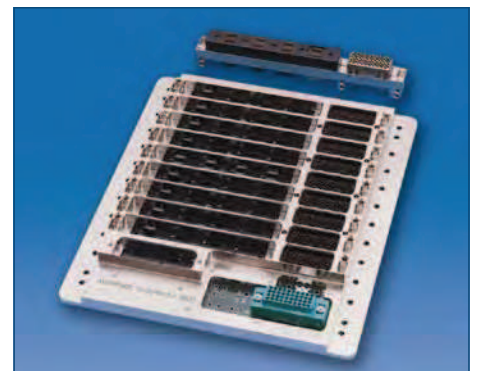
Backplane Incorporating LRM Modules with Brush Contacts and MT Fiber Optic Inserts
